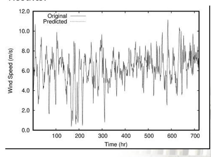
Actual wind speed time series at 80m height at Malambuzha (Palakkad District) in comparison with the corresponding values predicted using the wind data at 50m height at the same location by employing the prediction model trained with wind data at 80m and 50m heights from Kulathumedu (Idukki District).
