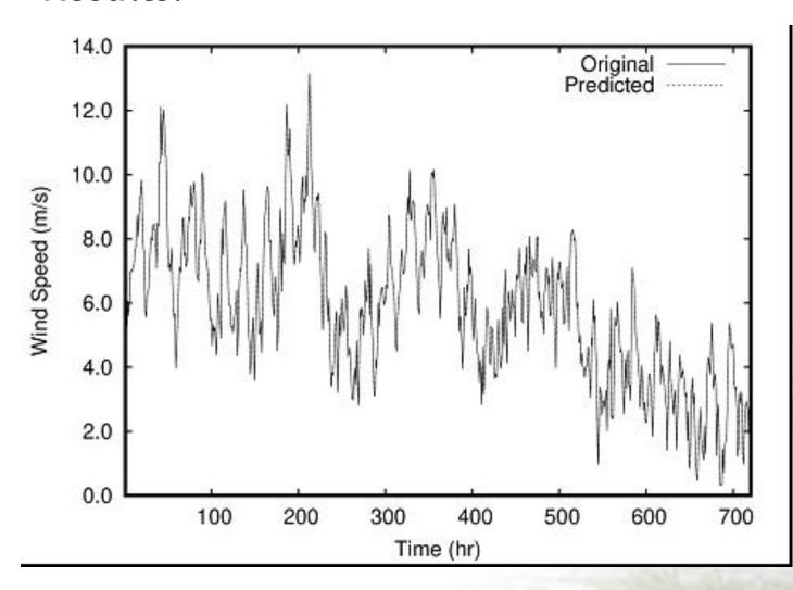
Actual wind speed time series at 80m height at Kulathumedu (Idukki District) in comparison with the corresponding values predicted using the wind data at 50m height at the same location by employing the prediction model trained with wind data at 80m and 50m heights from Malambuzha (Palakkad District).
