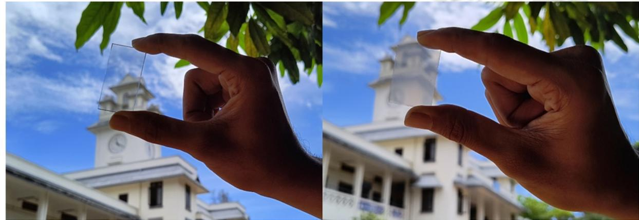
Photos of different substrates a) Photo of a  $5 \times 2.5 \text{ cm}^2$  commercial FTO substrate b) Photo of an in-house optimized FTO substrate ( $4.5 \times 2.5 \text{ cm}^2$ ).
