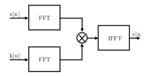
3. Segment the signal values into blocks of length N = 2000. Pad the last
