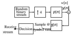
• Add AWGN (*w*[*n*]) of different variances and compute the BER-SNR curve for the bit patterns received.
