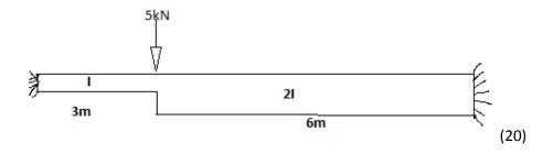
II) Analyse the frame by the method of consistent deformation and draw the BMD and SFD.
