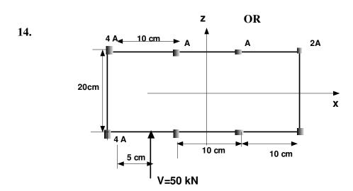
Obtain the shear flow distribution around a closed section subjected to a shear load V=50kN as shown in figure below. Stringer areas A= 6.24 sq. cm.
