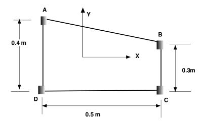
The above cantilever section is acted upon by two forces 10 kN along the Y-axis and 5 Kn along the x-axis at a distance of 1m from the fixed end. Determine the maximum bending stress in the boom stringers and the inclination of the neutral axes.
