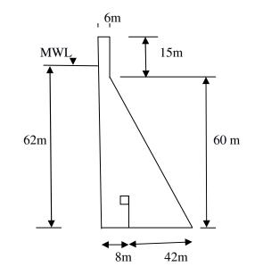
Check the stability of the gravity dam shown in the figure above for reservoir full condition. Assume co-efficient of friction =0.75. Consider only the weight of dam, Water pressure and uplift pressure. Take average shear strength q = 1.4N/mm<sup>2</sup> and density of concrete 24 kN/m<sup>3</sup>. Design a constant angle arch dam by thick cylinder theory for a valley with bottom width 50m and top width of 250m at a height of 100 m. Permissible stress is 5000kN/m<sup>2</sup>
